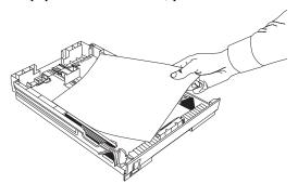
Note: Be sure the paper is under the tabs at the left and right edges of the cassette. Do not fill past the Paper Full marker. If necessary, readjust the guides for a snug (but not tight) fit.
